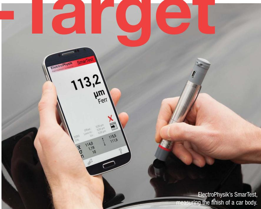
ElectroPhysik's SmarTest, measuring the finish of a car body.
