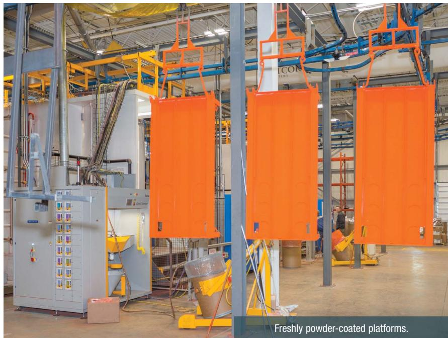
through a system of pinholes, so that more than 90 percent of what isn't applied directly to the substrate can be recaptured. The result is that the booth stays clean while, of course, powder usage is reduced.
