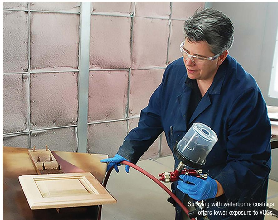
Spraying with waterborne coatings offers lower exposure to VOCs.
