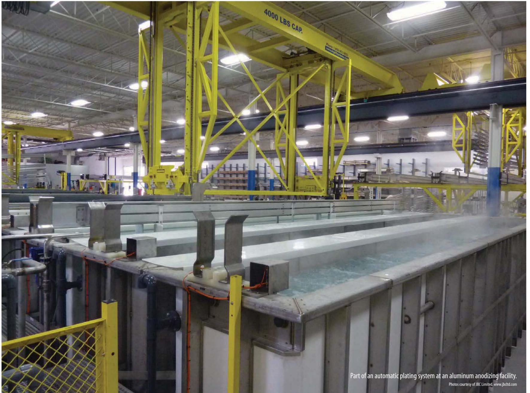
Part of an automatic plating system at an aluminum anodizing facility.
