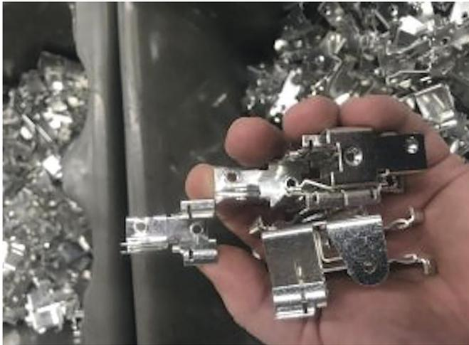
TECHNIBRITE SN 200 tin process provides lustrous, bright tin deposits.
